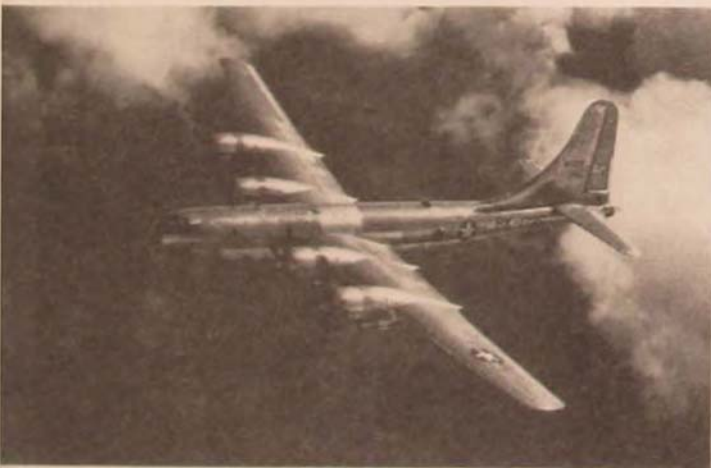
The piston-powered bombers of the forties dominated the post-World War II era. The B-29 Superfortress (left) was much used in the Pacific at the end of the war and was the USAF's first nuclear delivery vehicle. . . . Early follow-ons were the world's largest aircraft, the B-36 (top), shown in its August 1946 first flight, and the B-50A (above), a more efficient modification of the B-29.
