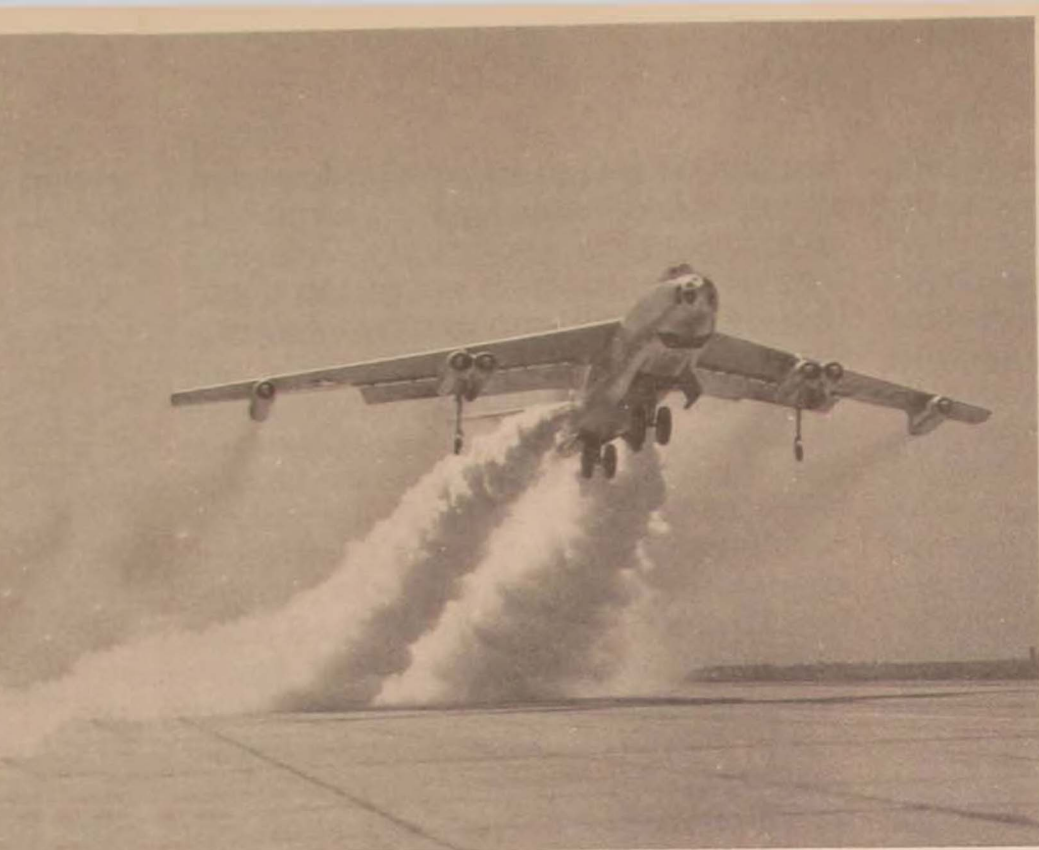
Jet-powered bombers came into their own in the 1950s with the B-47 Stratojet (left), and the B-52. The B-47, introduced in the late forties, is shown assisted in take-off by its 18 rocket units. The B-52 Stratofortress "Buff" shows the promise of being as indestructible as the venerable C-47.
